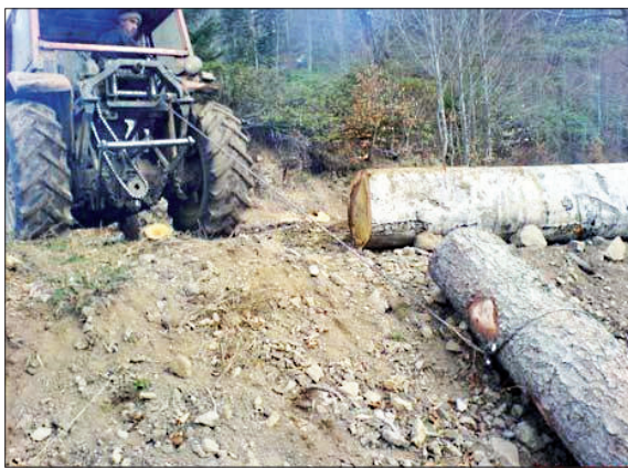
Figure 1. Cable winching (left) and skidding (right) with farm tractor
