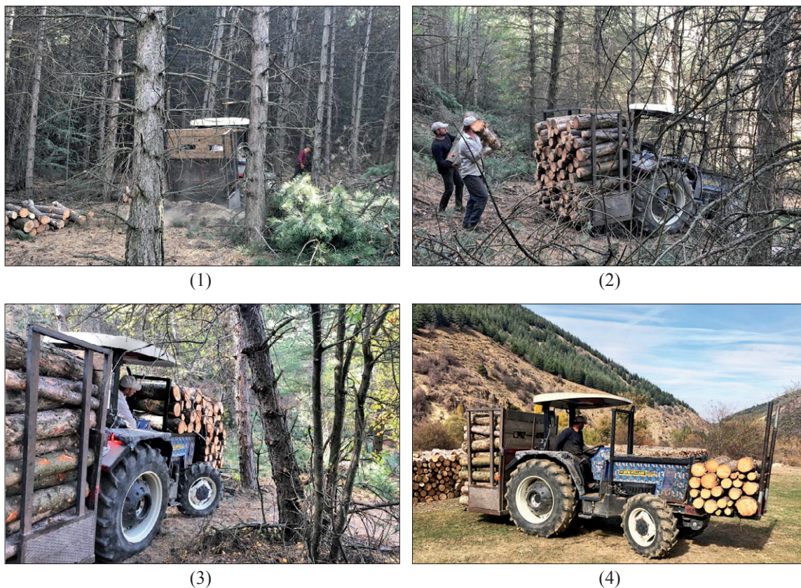
Figure 4. The work stages of the tractor skidding: 1) the unloaded tractor to reach the point where the wood products are located; 2) collect and load the products at the stump; 3) the time of the loaded tractor to reach the landing area; 4) the time of unloading tractor and stacking the wood products at the landing.
