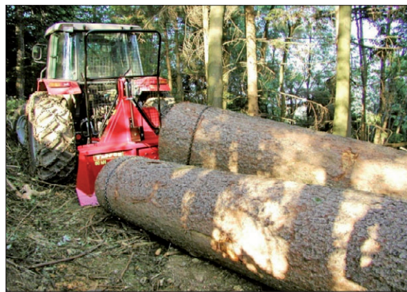
Figure 1. Cable winching (left) and skidding (right) with farm tractor
