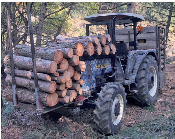
Figure 2. Extracting stere woods with a saddle attached to the tractor
